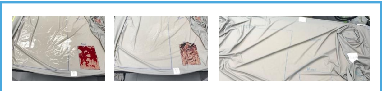
(a) Soil on barrier before laundering. (b) Dried soil on barrier before laundering. (c) Barrier surface completely clean of soil after laundering.
