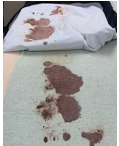
Image 3: Staining on bottom of integrated mattress cover and top of fire barrier
