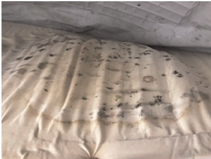
Image 5: Blood and bodily fluid ingress contaminating internal components. 9
